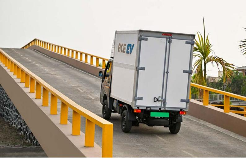
The vehicle supports a regular and fast charging system. The EV can be charged via a standard 15A socket in a home environment. When a regular charger is used, 20% to 100% charging can be achieved in 6-7 hours. Whereas the Ace EV can be charged up to 10% to 80% charging in 105 minutes with a fast charger.
