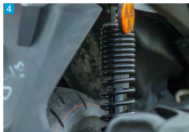
1. Buttons to open the seat and fuel cap 2. LED Headlights 3. VVA - Variable Valve Actuation Technology 4. Twin shock absorbers at the rear
