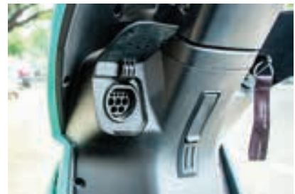
It takes nearly 5.45 hours to charge the battery to 100 percent by wall mounted charger
